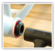
2. Insert the left side adapter. Spacers can be placed on either side to center cranks in bottom bracket.
