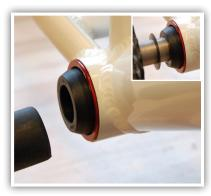
1. Insert the right side adapter into BB30 or PF30 Bottom bracket by hand. Note: BB30 and PF30 dust covers can be removed from the system or left in place. If you choose to use them with the BBUNIV-SHIM, place them between the bearing and the adapters on both sides. Right side spacers (24mm I.D.) fit on the BB spindle between the right side adapter and the right crank arm.
