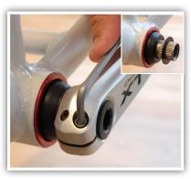
3. Install the crank. If there is side-to-side play, you may need 24 mm spacer(s) on the outside and/or additional 30 mm spacer(s) installed on the inside of the adapter. Tighten to manufacturer's specification. Crank should spin freely.
